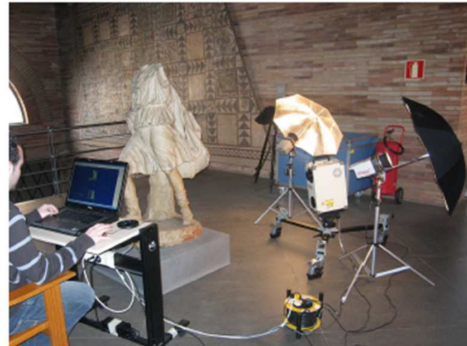
Figure 6. Moment of the scanning of Ascanius in the MNAR. The picture shows the lighting system used and the scanner mounted on a dolly.
